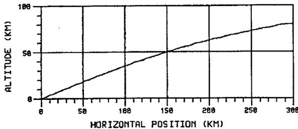
Figure 5. Altitude versus horizontal distance for a typical incline section.
