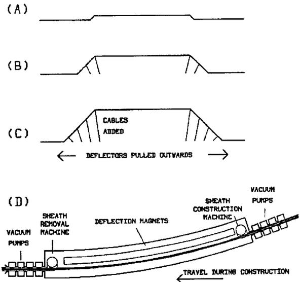
Figure 11. Starting up the Launch Loop. (a) up to speed, flat on the surface. (b) partially raised, with the ramps pulling towards the ends. (c) fully erected, the track sheath being stripped away. (d) the west end incline deflector during erection.
