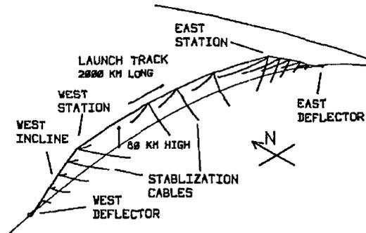
Fig. 1. A side view of the Launch Loop. Most cross sections are in centimeters, making the structure virtually invisible from a distance.
