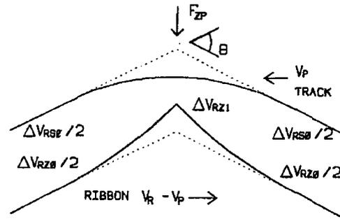
Fig. 9. The deflection of ribbon and track as they pass by the vehicle.
