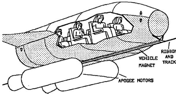
Fig. 8. A typical 5 ton passenger vehicle, with magnets, rocket motors for apogee orbit insertion and a heat shield for accidental reentry.
