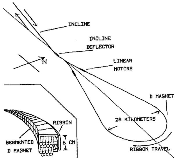
Figure 4. The east end deflectors, motors, and the start of the east incline. The inset shows a section of deflector magnet.
