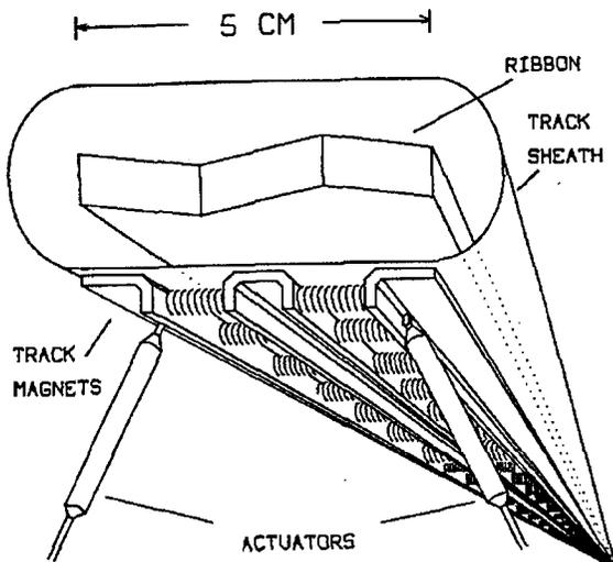
Fig. 2. A cross section of the ribbon and track.
