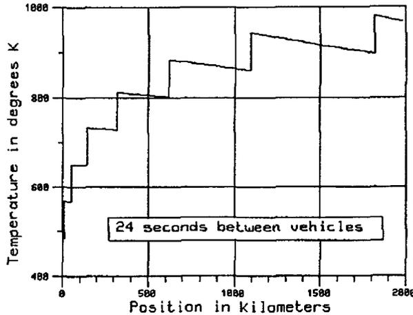
Figure 10. Temperature profile of the Launch Loop ribbon during a burst launch.
