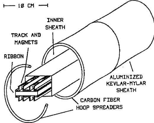
Fig. 6. Cross section of the incline sheath
