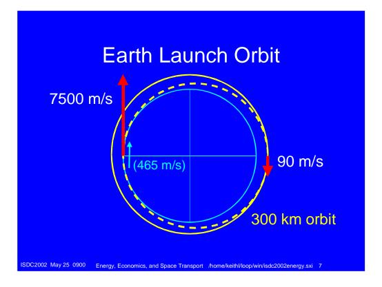
Launching from the equator adds the rotation speed of 460 meters per second to all launches.
