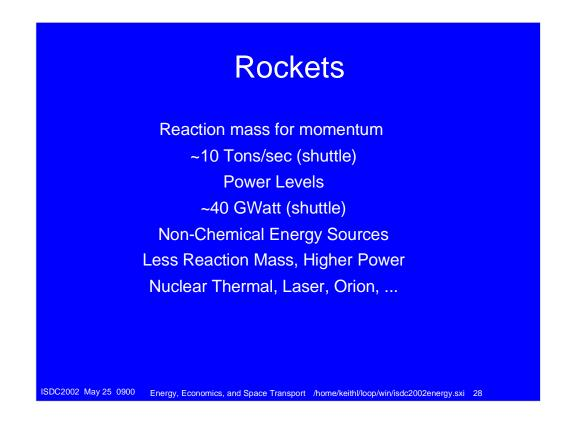
Rockets are self contained. They provide their own energy and reaction mass. At launch, the space shuttle is producing over 10 tons of exhaust per second, with a power level of 10 billion watts.
