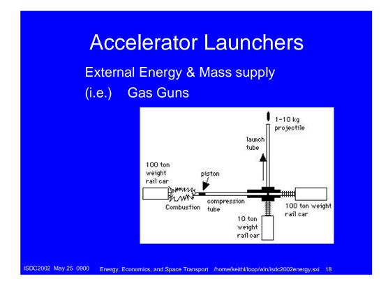
The next few slides will present some accelerator launchers. These get around the "rocket problem" by using both external energy sources and external reaction mass. Thus, we bypass the exponential scaling of rocket systems. The classical accelerator launcher is the cannon, and its modern equivalent is the gas gun. Gas guns produce a stream of very high energy hydrogen that pushes small payloads to high speeds. However, we have not made one yet that can reach orbital velocity.
