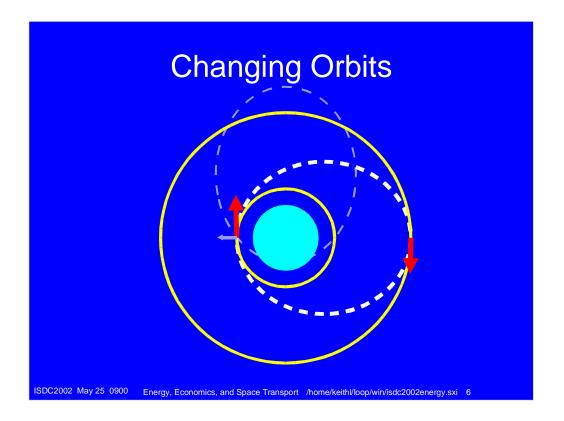
To get from anywhere to anywhere else involves changing orbits. To go from a low circular orbit to a high one involves two velocity changes, one <u>HERE</u> that puts you into an elliptical transfer orbit, and one <u>OUT HERE</u> that takes you out of the elliptical transfer orbit and injects you into a circular orbit.
