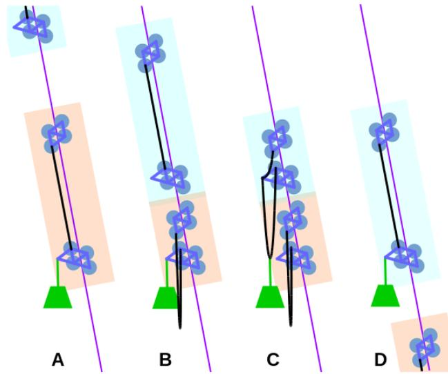
Figure 16: **Transferring payload from a lower to an upper acoustic climber**
