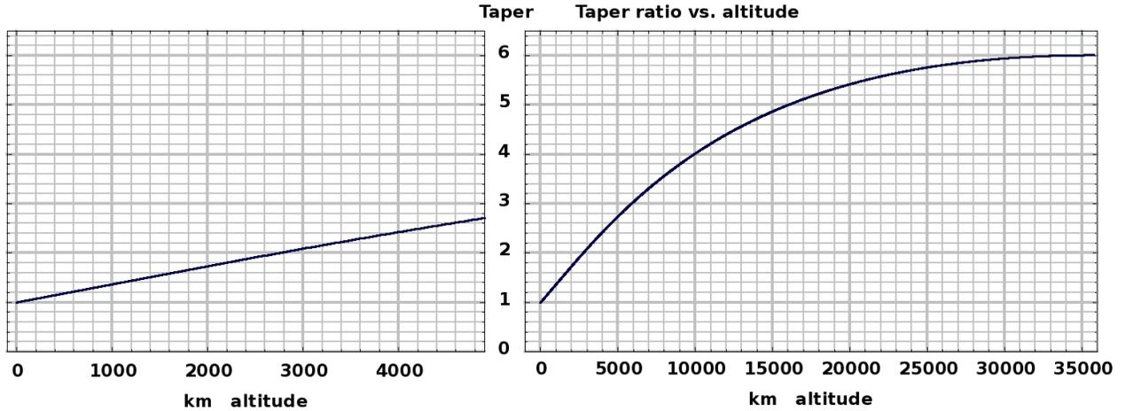
Figure 10: **Tether taper versus altitude.** Reduced gravity at higher altitudes reduces the rate of taper increase.
