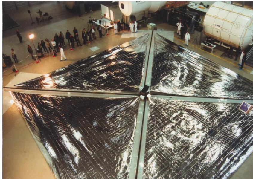
Figure 1: 2003 DLR/ESA 400 m<sup>2</sup> solar sail prototype
