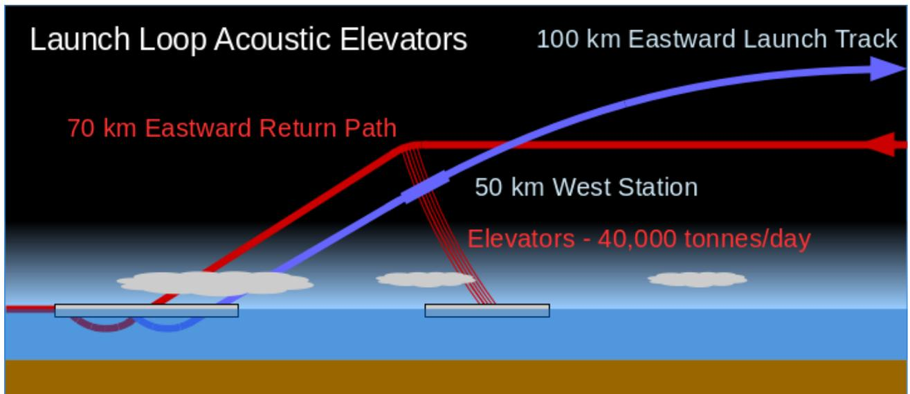
Figure 18: Launch loop elevator system. Dozens of Kevlar elevators carry 7 tonne acoustic climber vehicles from the surface to the West station of the launch loop, where the launch vehicles are tested then propelled up the launch track.
