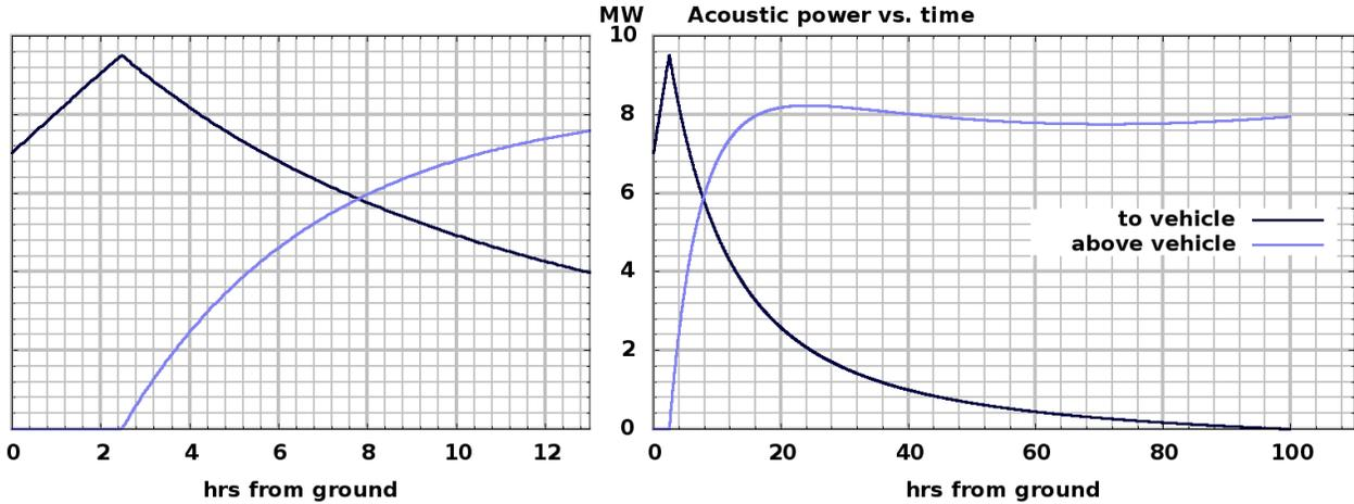
Figure 15: **Power used by a 16 tonne vehicle vs. time** Ascent speed limited to 100 m/s, or by available power.
