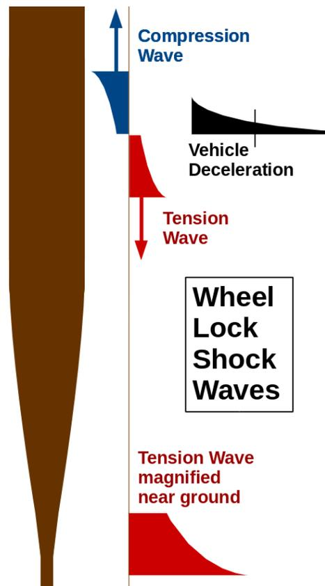
Figure 3: **Wheel shockwaves.** A failed wheel may lock up or fracture, and suddenly stop on the tether. This launches huge stress waves down the tether.
