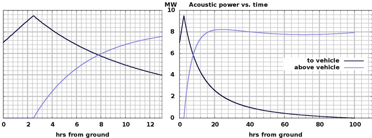
Figure 12: **Power vs. time, single vehicle on the tether** One vehicle on the tether. The assumed top speed is 100m/s for a 16 tonne vehicle. These numbers will increase greatly at middle altitudes when an acoustic transmitter is added at GEO.
