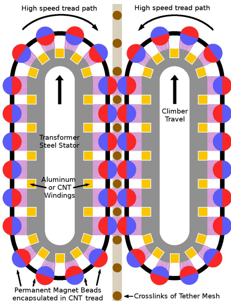
Figure 4: Magnetread climber "wheels"
