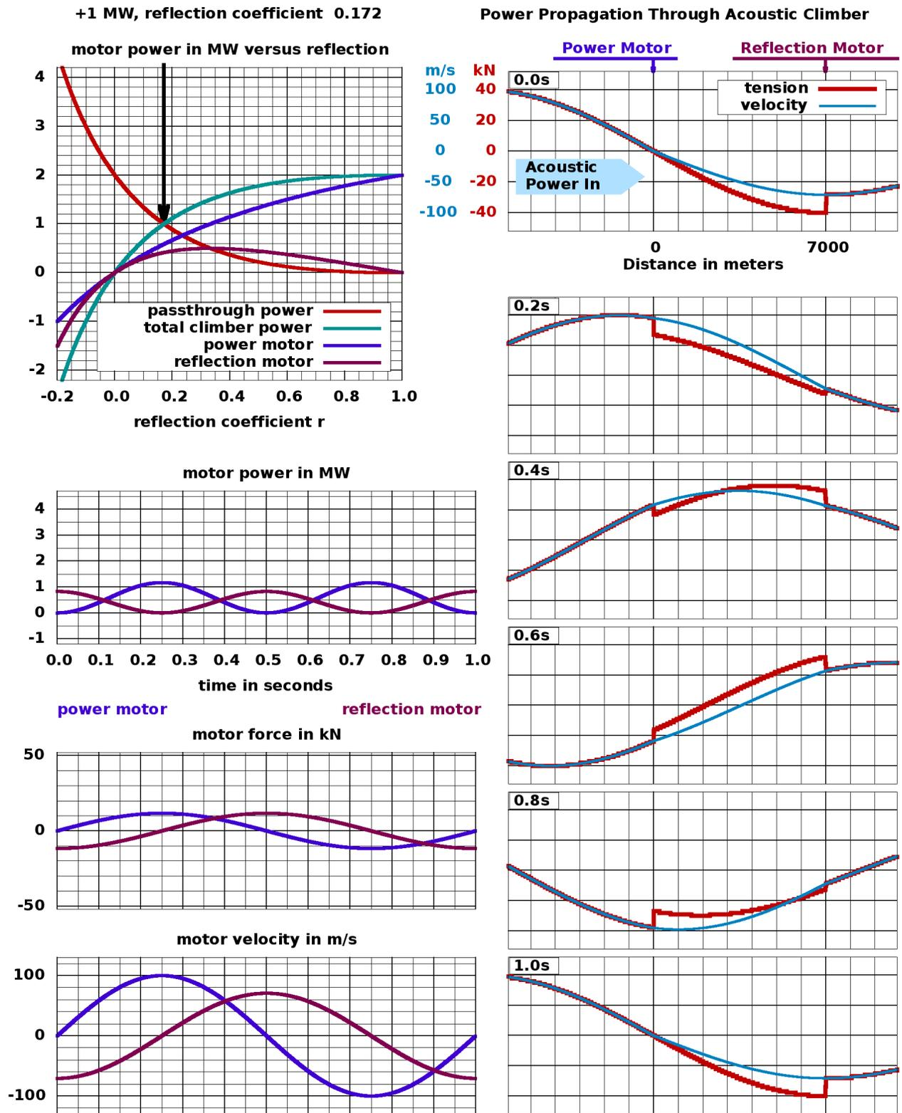
Figure 8: 1 MW power absorbed; using half of the power arriving at the climber.
