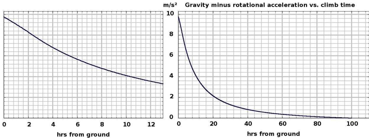
Figure 11: **Gravity (minus centripetal acceleration) versus altitude**
