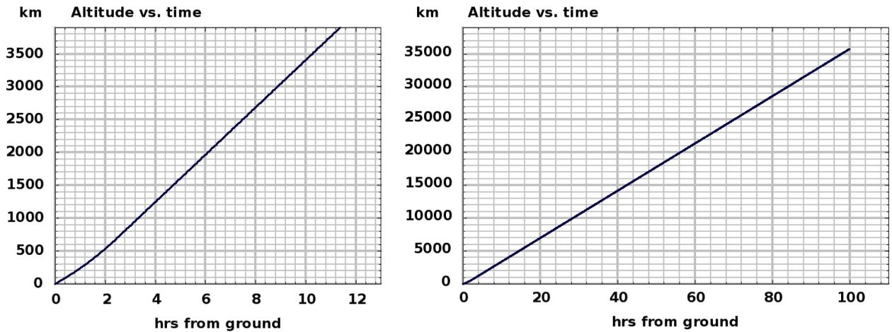
Figure 14: **Altitude versus climb time.** After 12 hours, the vehicle climbs at full speed.
