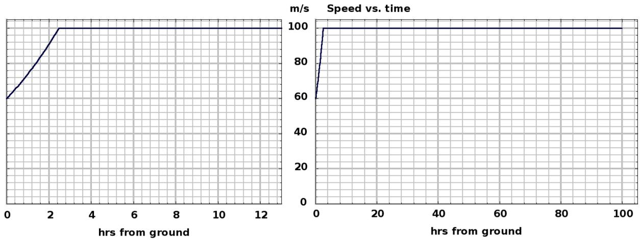
Figure 13: **Speed versus time, single vehicle on tether.** Speed is proportional to power divided by gravity and the 16 tonne vehicle mass. The maximum climb speed is presumed to be limited to 100 m/s. Below 400 km altitude, climb speed is power limited. Multiple vehicles on the tether reduces the surplus tension available beneath the vehicle to accommodate acoustic power.
