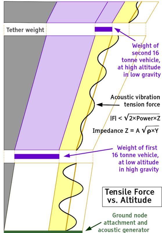
Figure 17: Tether tension versus altitude
