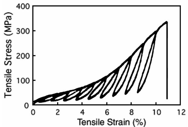
Figure 2: Weakness, Hysteresis, Creep, and Failure for a CNT Yarn
