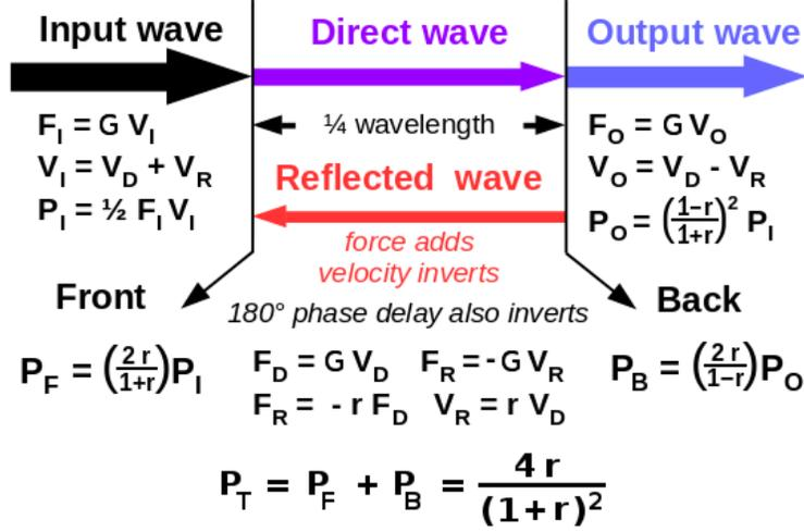
Figure 7: Acoustic receiver velocity, force and power
