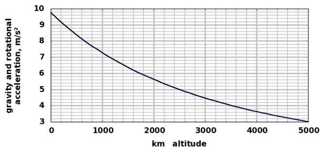
Fig. 6. Gravity minus centrifugal acceleration versus altitude
